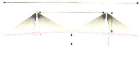
This cable stay bridge has 20 *cables*. The *deck* of the bridge is *1.2 km* long, and is *18 m* above water level. Each *pier* is *35 m* wide. The *span* between the two pylons is *832 m* long. Each pylon is *45 m* high above the road deck.
