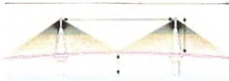
This cable-stay bridge has 20 *cables*. The *deck* of the bridge is 1.2 *km* long, and is 185 *m* above water level. Each *pier* is 35 *m* wide. The *span* between the two piers is 832 *m* long. Each *pylon* is 45 *m* high above the road deck.
