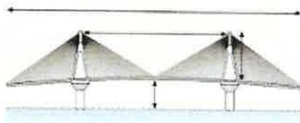
This cable-stay bridge has 20 cables. The deck of the bridge is 1.2 km long, and is 185 m above water level. Each pier is 35 m wide. The span between the two piers is 832 m long. Each pylon is 45 m high above the road deck.
